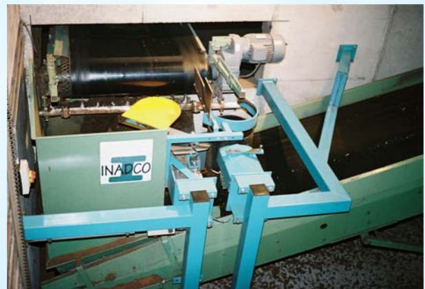
The yellow shovel takes samples from the belt and drops them in the black CEN Measuring Cylinder (with white bottom).
